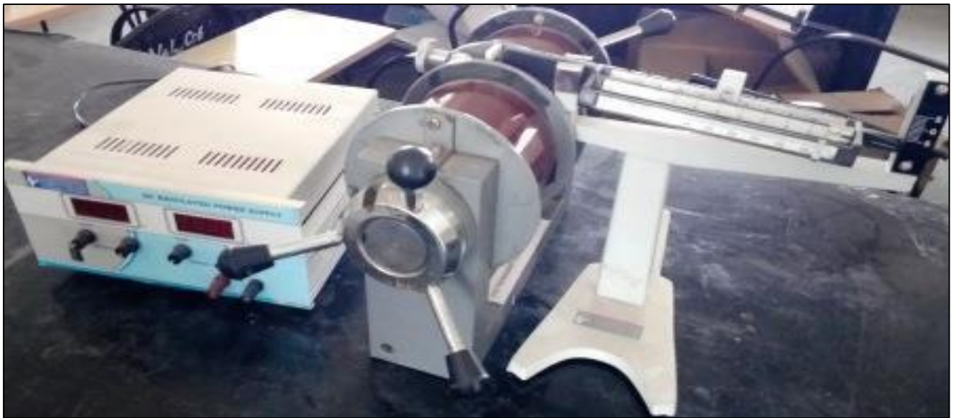
Susceptibility measurement for solids by Guoy's method
